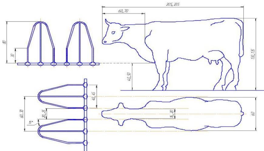
Figure 3: Dimensions of the separation grid
